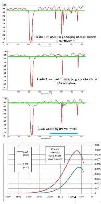
These black body graphs show emissions at typical temperatures of the black foam board at the back of the \_\_\_\_\_ boxes. Emissions at these wave numbers are incident on the covering materials. The red transmission spectra give the percent of the incident emissions that get through.
