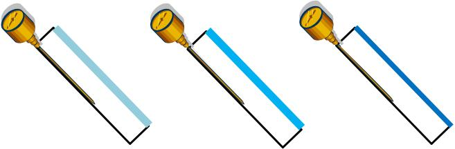
I stuck a cooking thermometer in each box to measure the temperature near the black material lining the bottom (black foam board). The thermometers themselves reside inside of a reflective metal tube (I took one apart and checked). They are not in direct sunlight. The tubes are designed to be stuck into a hunk of meat being cooked, but they served the purpose here. (I'm retired. I use what I find.)
