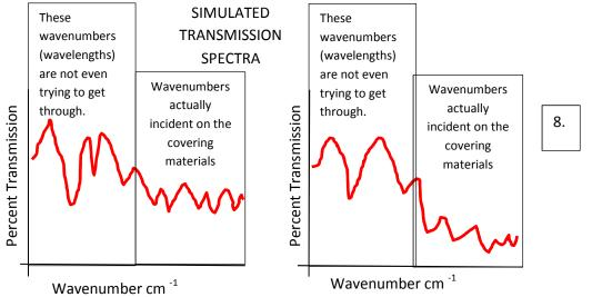
It was possible to qualitatively notice which covering material was transmitting more and which less. Here the right-hand material is transmitting less and thus trapping more infrared at least in the wavenumber range actually used. (Panels 6, 8)
