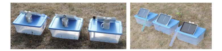
Boxes used here for the first set of trials and platforms for holding them. Notice the control box with no cover (extreme right). The 30-cm rulers show the scale. Sometimes paper stuffing was necessary to keep the thermometers touching the bottom. They measured 3 cm x 16 cm x 24 cm. Notice the drought conditions, which at least gave me a lot of days of weather that was good for this project.
